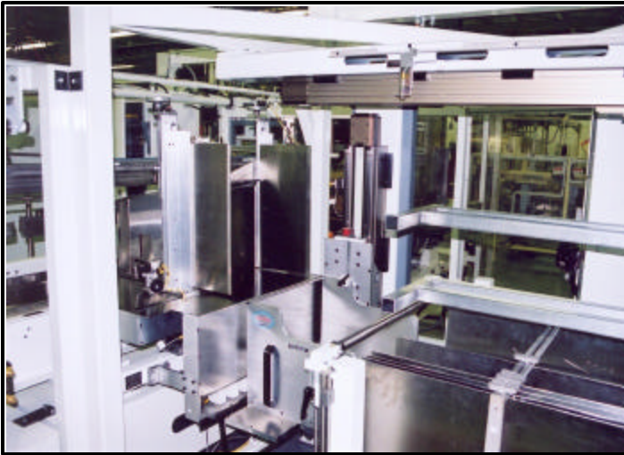
Guarding removed for clarity – note extra size range capability of stainless steel deck and sensor board already built it.
