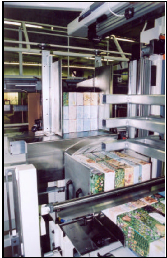
Facial cartons being inducted into cassette; full case load is accumulated in retractable chute
