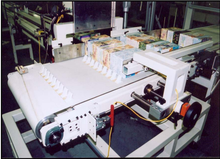
Guarding removed – note convenient backstop adjustment
